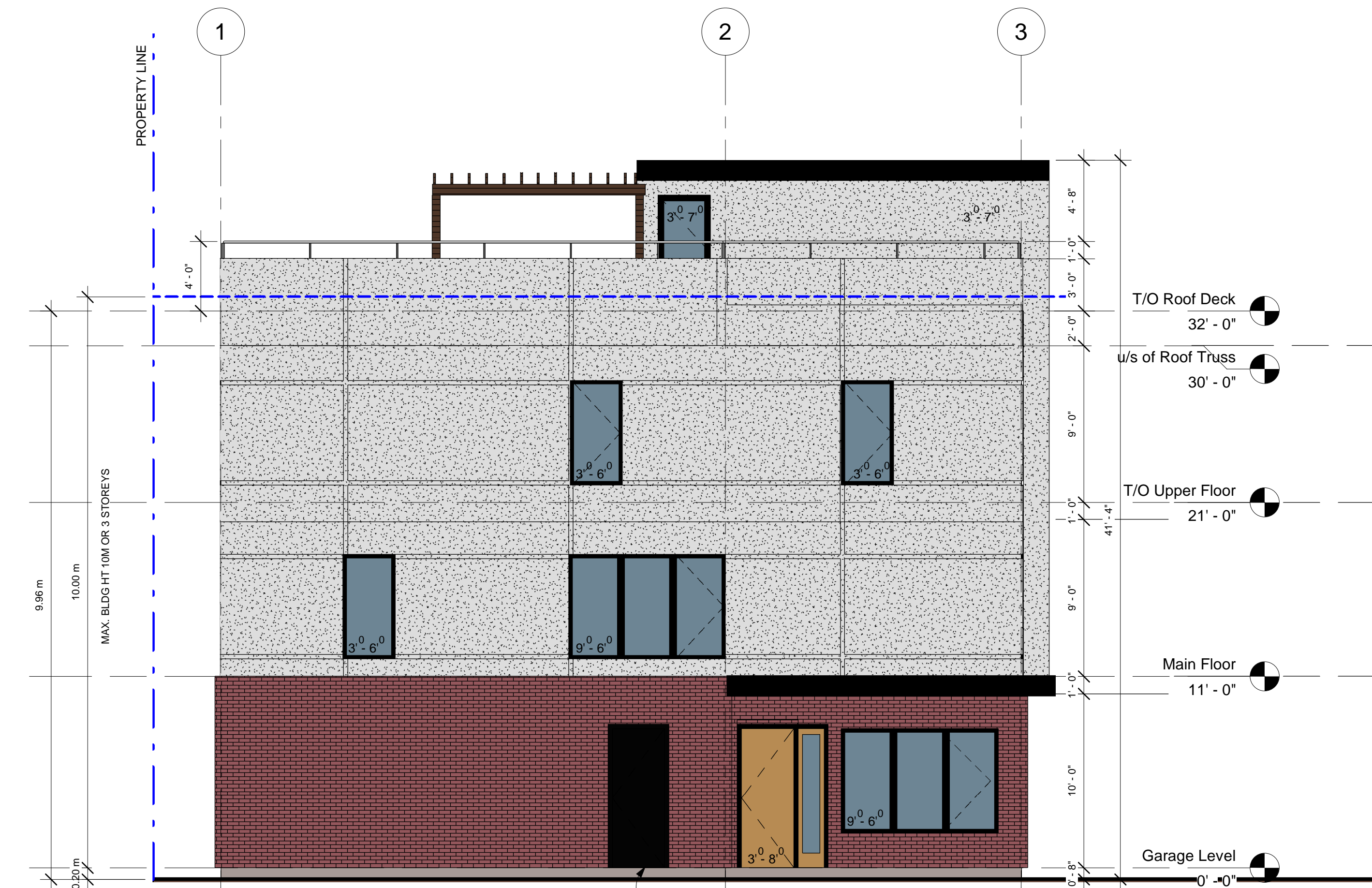
1 BLDG 1 - East Elevation (Mallach Rd.) 3/16" = 1'-0"
