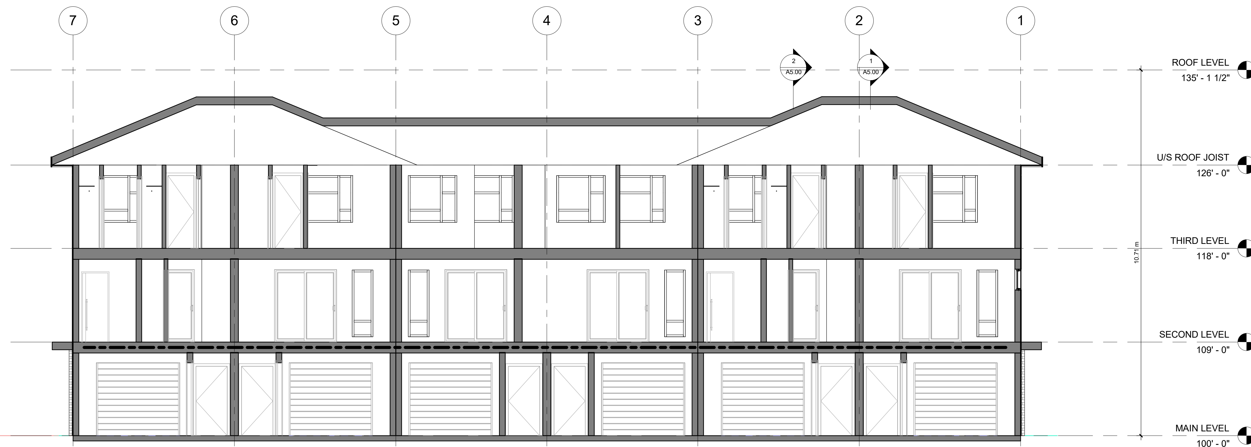
3 BUILDING SECTION - 6 UNIT BUILDING A3.01 3/16" = 1'-0"
