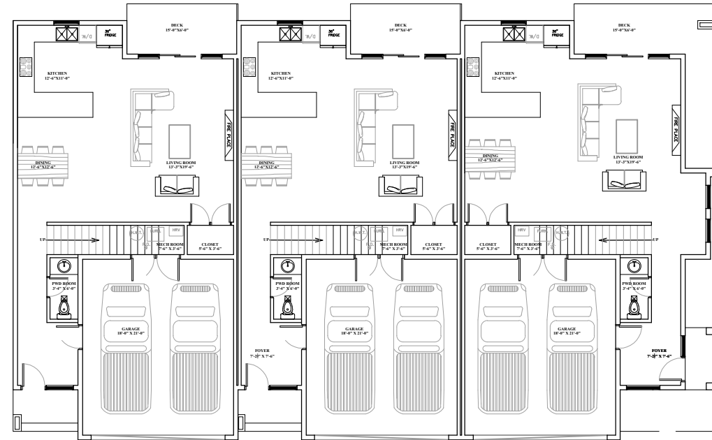
MAIN FLOOR PLAN B-1 SCALE: 1/16" = 1'-0" PROPOSED FLOOR : 860.74 SQ. FT. PER DU GARAGE: 378 SQ. FT. EACH
