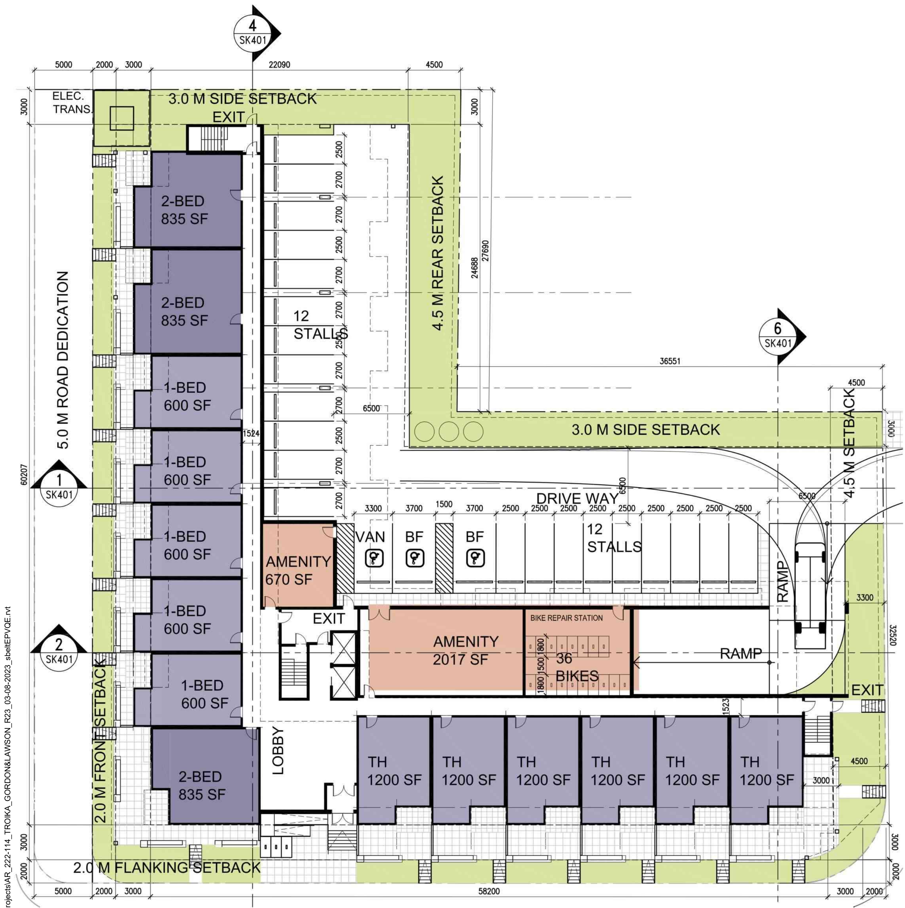
GROUND FLOOR PLAN SCALE: 1:200
