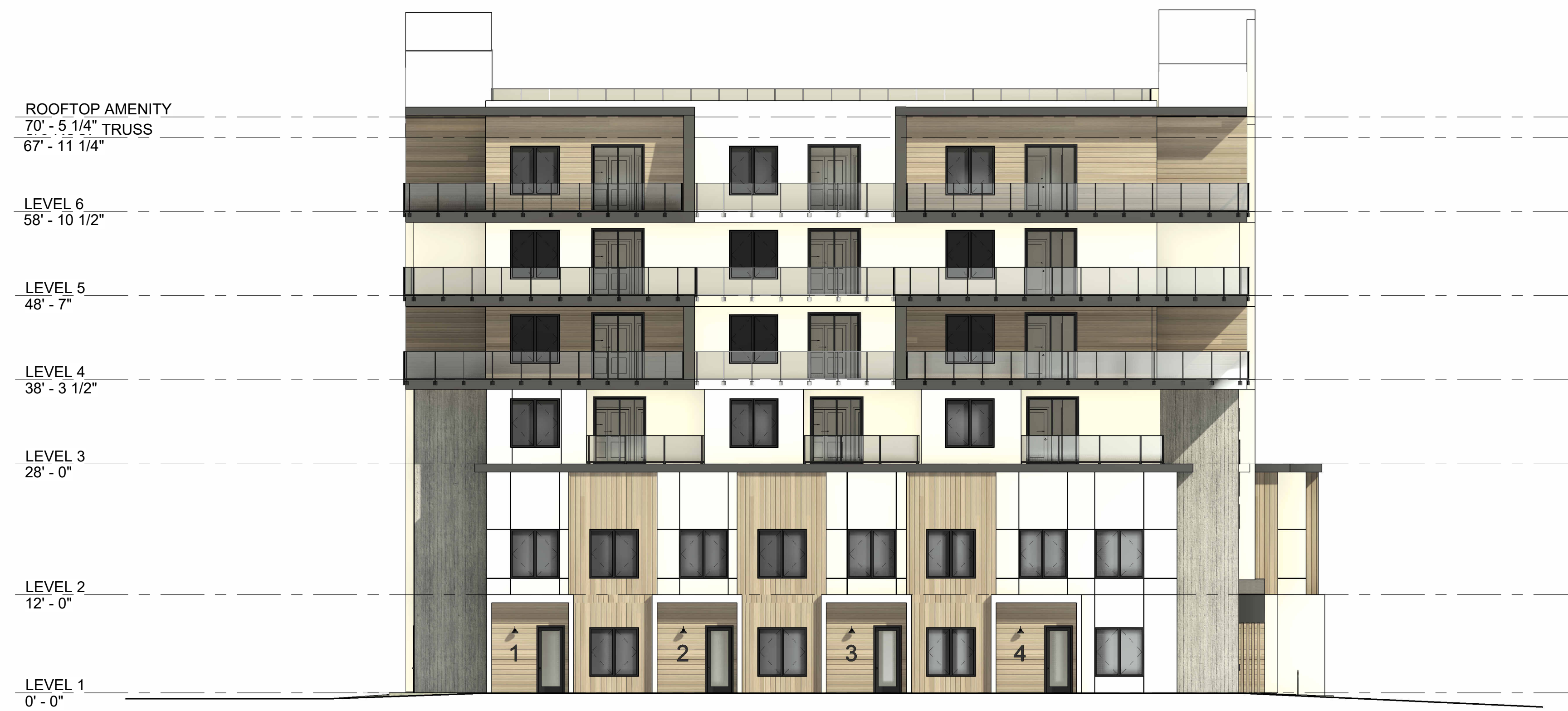
2 EAST ELEVATION (COLORED) A-201 3/32" = 1'-0"
