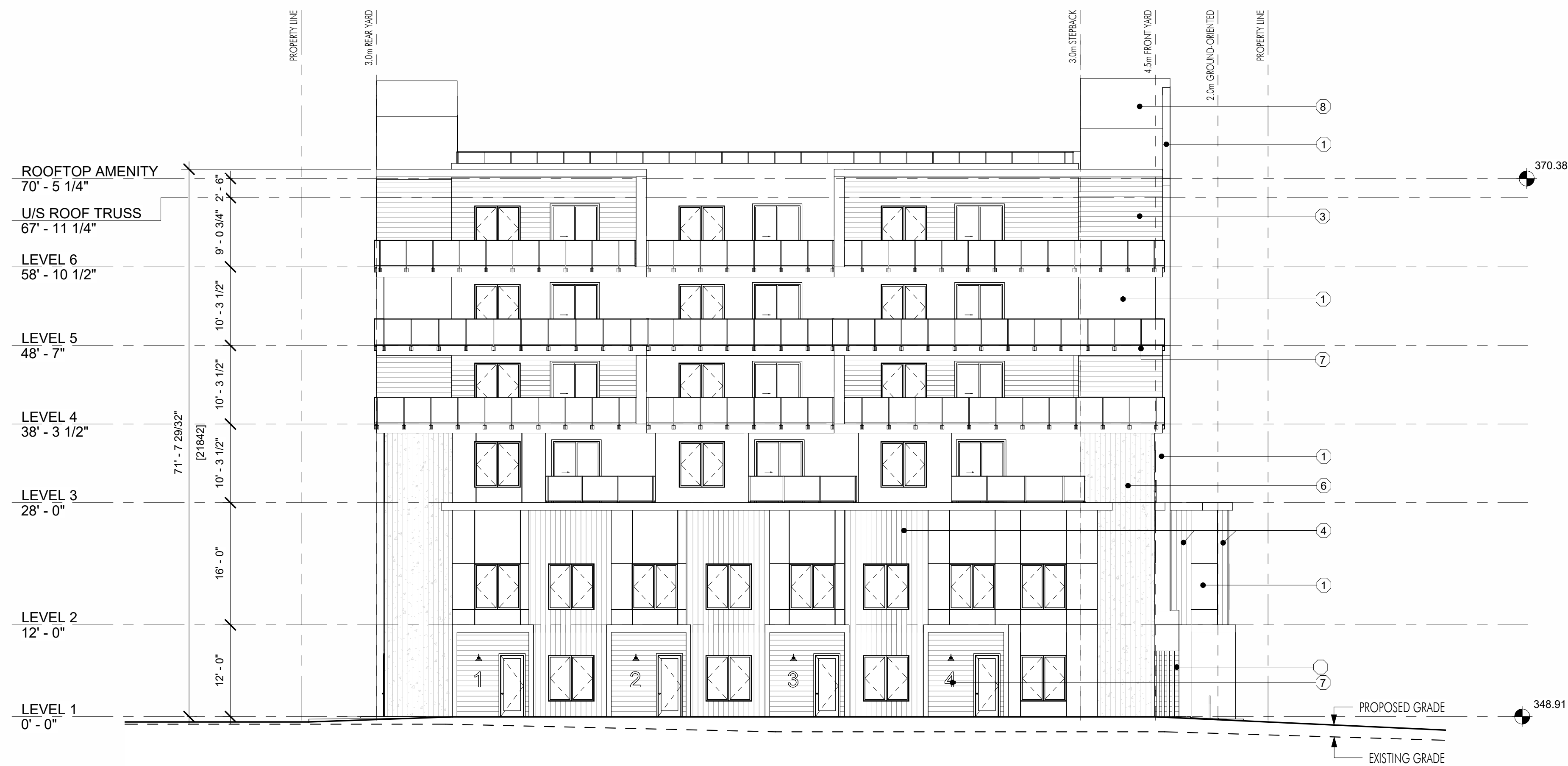
1 EAST ELEVATION A-201 3/32" = 1'-0"
