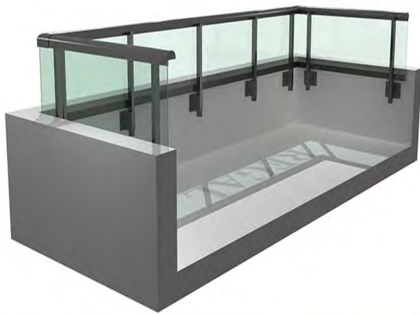
BALCONY RAILING SYSTEM @ L6
