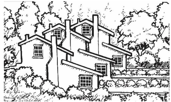
Figure 19.2: Step buildings up or down the slope
